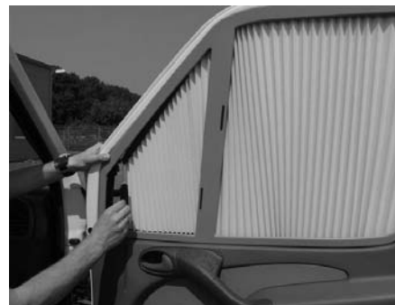
C5: Bring handle up to stop rail, magnetic catch locks automatically.
