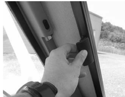
C1: Push button up to unlock front blind.
