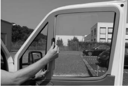
B34: Insert frame and press against door.
