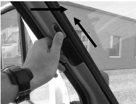
C1: Push button up to unlock front blind.
