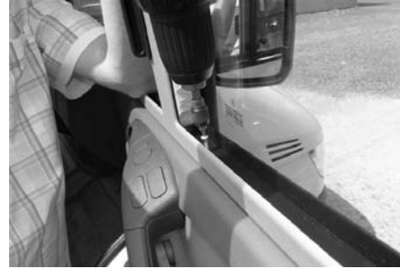
B34: Insert frame and press against door.
