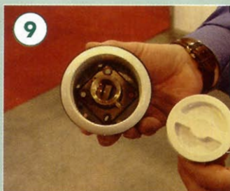
9. The white or black UK Autogas bayonet-type filler units are sold complete with installation fixings
