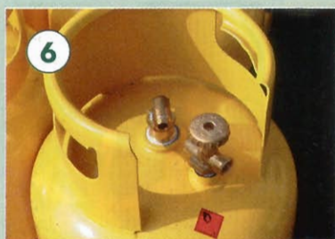
6. The supply outlet to the caravan is the screw type fitted on Calor 4.5kg butane cylinders
