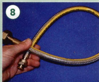
8. Though not as flexible as a standard rubber compound hose, this stainless steel pipe can be bent
