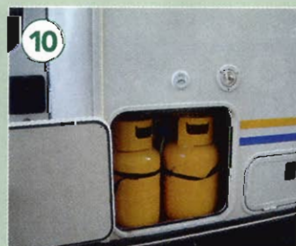
10. The wall-mounted filler on this motor caravan provides a safe and certain coupling point
